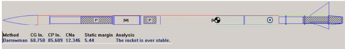
Figure 1: Diagram showing the stability of the rocket.
